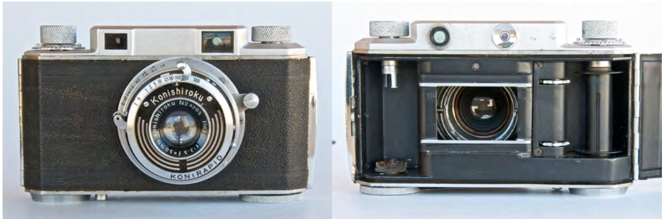
Fig. 14. Front and back of the first model Konica (late 1847) with black shutter face (Spennemann, 2011a).
