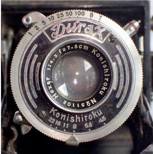
Fig. 4. Konishiroku Hexar 75mm f/4.5 in Durax shutter (in Semi-Pearl 4.5 x 6 roll film folder).
